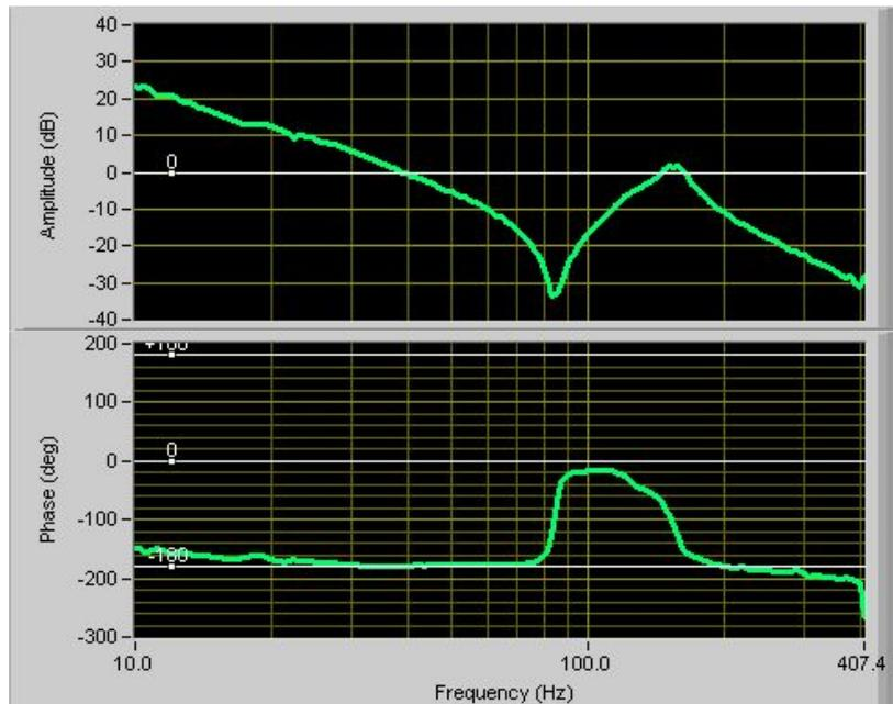
**Figure 14:** Plant FRF when Sensor is on the Motor
