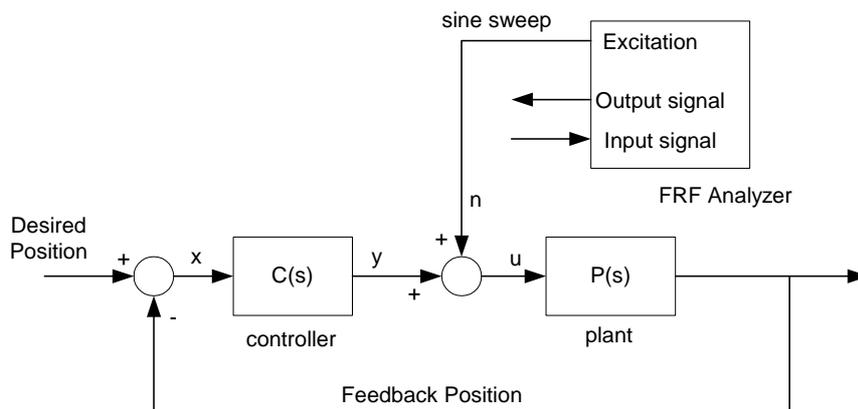
**Figure 2: FRF Measurement in a Closed-Loop**
