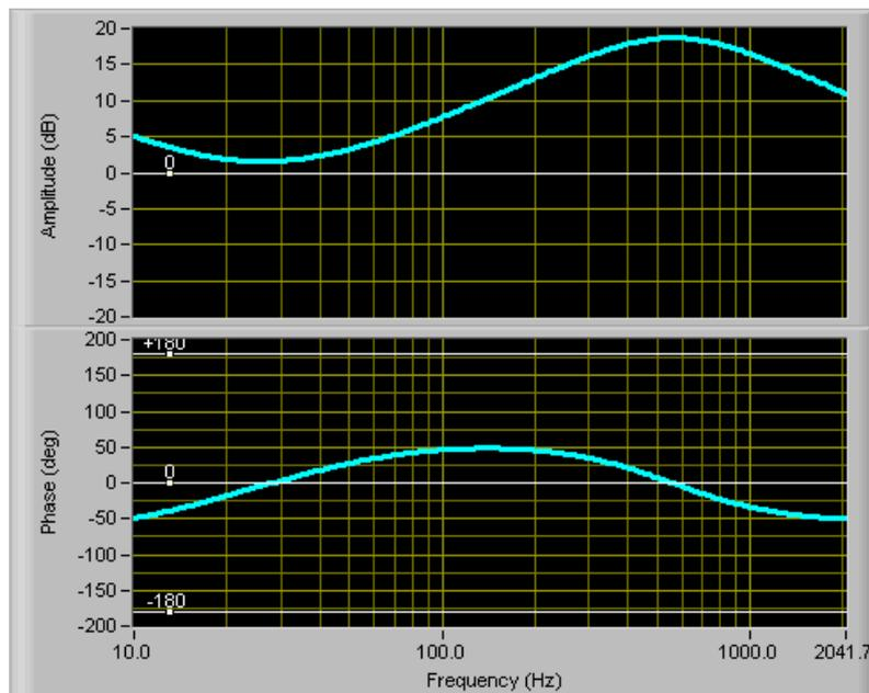
**Figure 7:** Controller FRF: PIV in Series with 2<sup>nd</sup> Order Low Pass Filter
