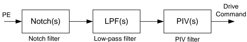
**Figure 6:** Equivalent Control Scheme
