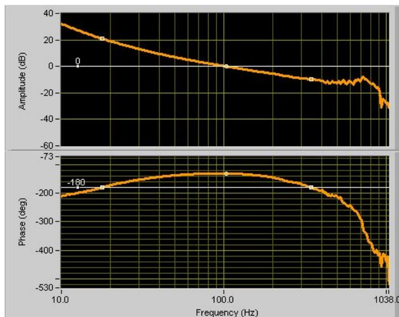
**Figure 8:** Open-Loop FRF
