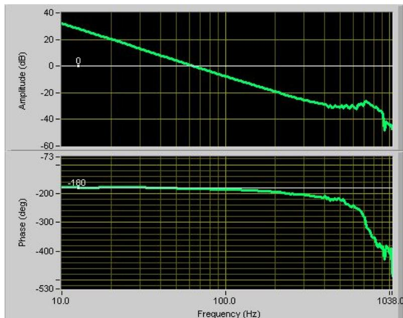
**Figure 4:** Simple Motor FRF
