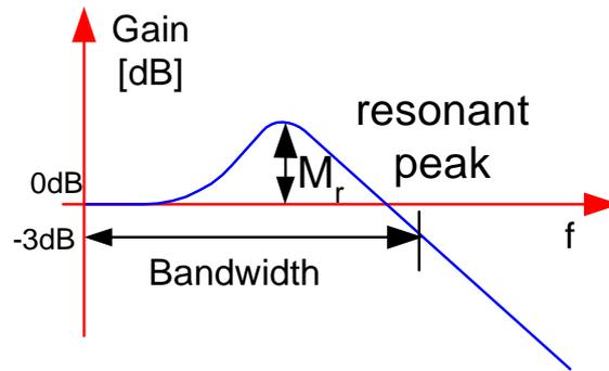
**Figure 11:** Resonant Peak Definition
