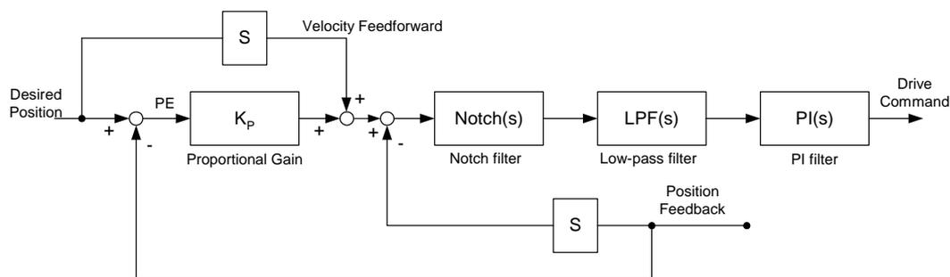
**Figure 5:** Basic Motion Control Scheme
