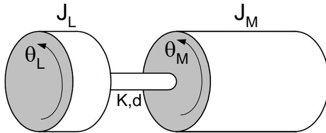
**Figure 12:** Compliantly Coupled Motor and Load
