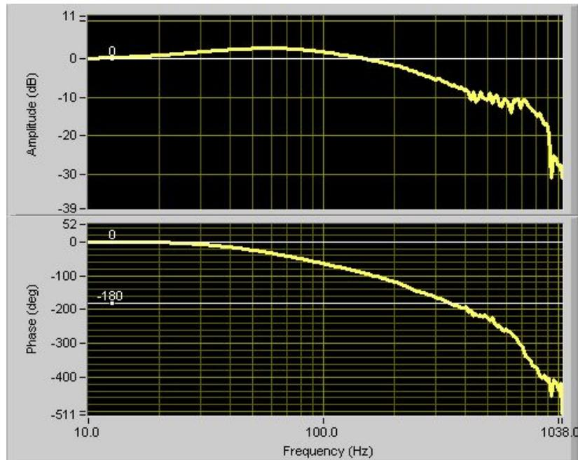
**Figure 9:** Closed Loop FRF
